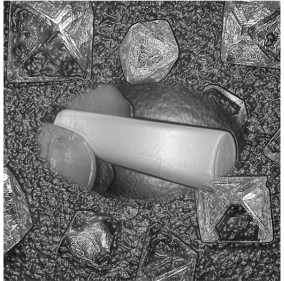
Cover Photograph: CaWO 4 crystals grown from chalk powders by flux method (Takahiko Ashizawa, Yamura Tech. High-school, p.83)
